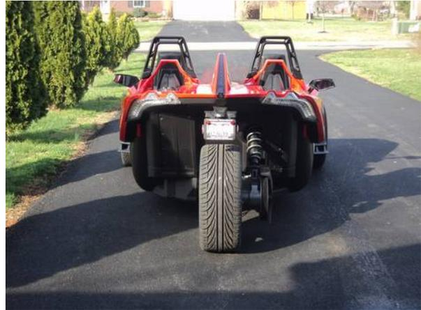
Here is what most riders see when the gas pedal is depressed (no twisting a throttle). A 2.4 liter GM engine and a 5 speed transmission makes it go.
